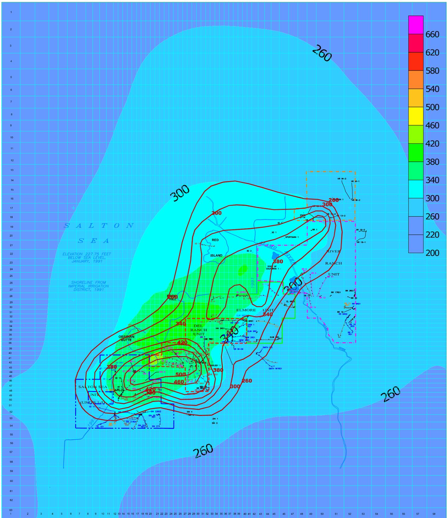
Figure 2.1 Matching of Subsurface Temperature at - 1,350 ft msl
