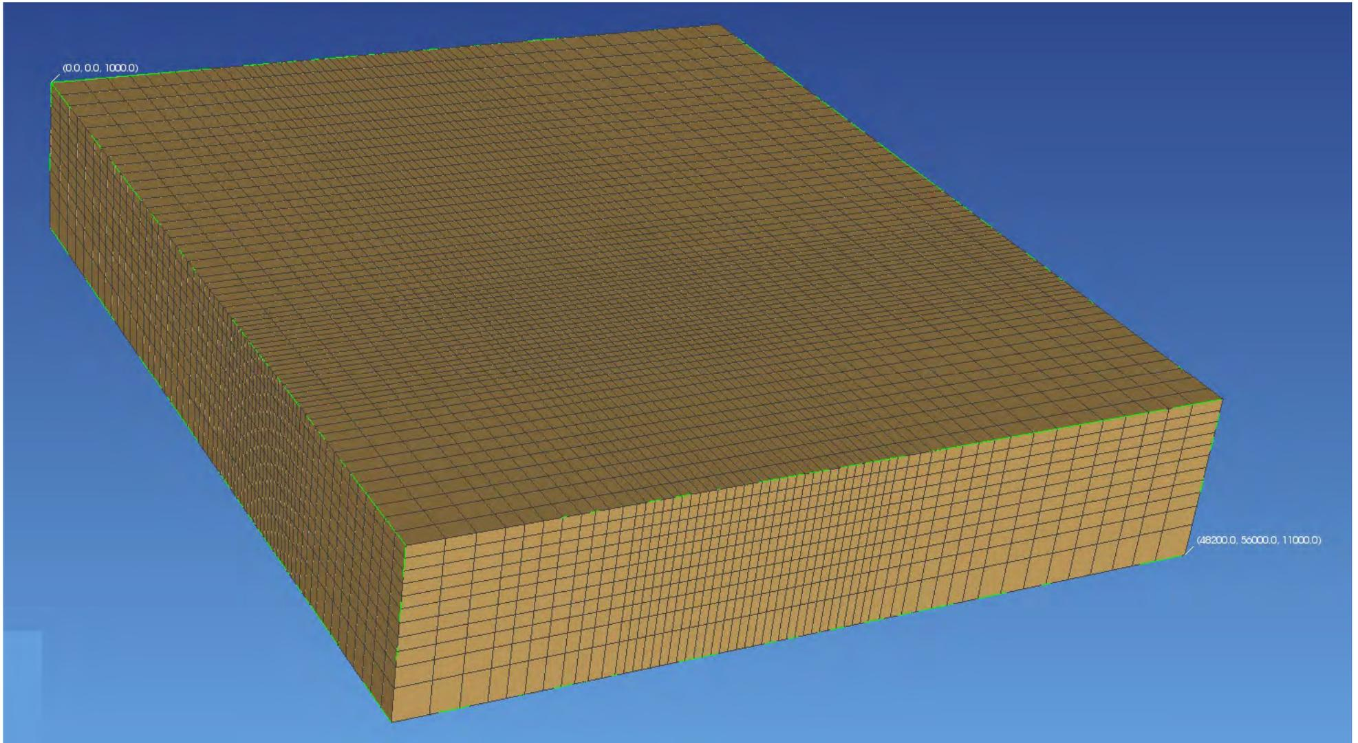
Figure 1.2 3-D View of the Salton Sea Numerical Model
