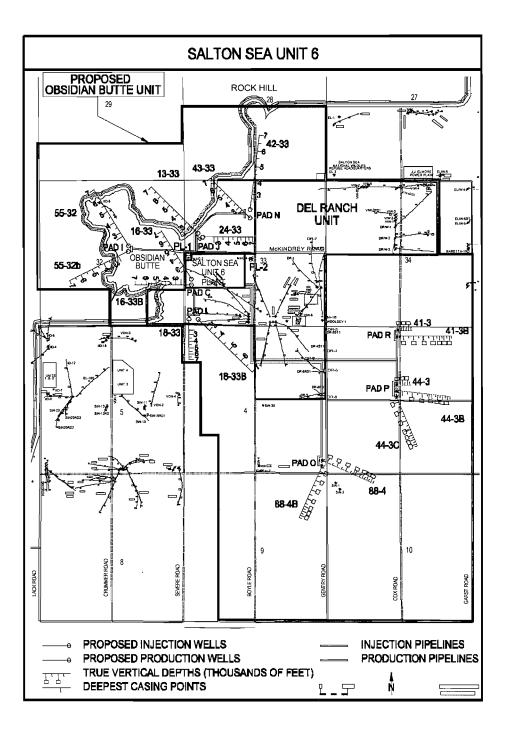
Figure 2: Proposed Unit 6 Wellfield Layout
