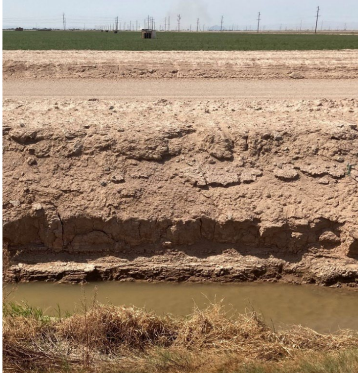
Photograph 1: Lake Cahuilla bed sediments exposed in the canal bank on the north side of Schrimpf Road. Facing south.
