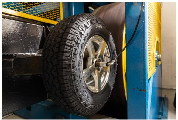
Photograph A5.6: Tire Ready for Testing
