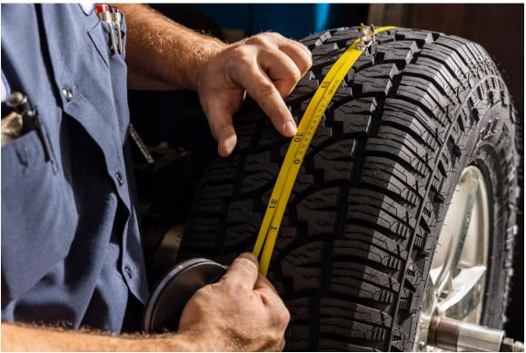
Photograph A5.5: Measuring Outside Diameter
