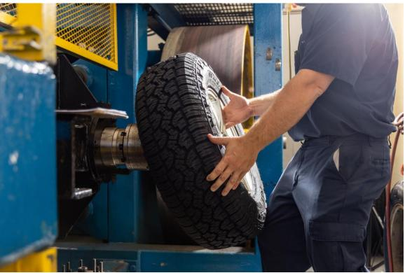
Photograph A5.1: Mounting Rolling Resistance Tire
