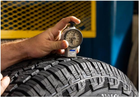
Photograph A5.3: Measuring Tread Hardness
