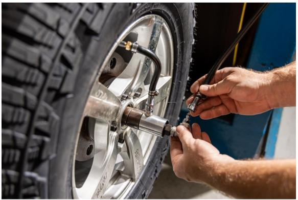
Photograph A5.2: Connecting Tire to Air Pressure
