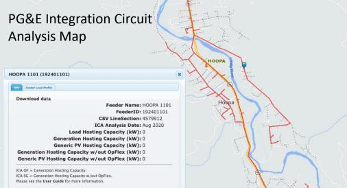
HOOPA 1101 circuit hosting capacity is **zero** across the board -- loads and generation. This is the same out to Wautec and Somes Bar. **Outages are frequent**: PSPS, storms, landslides, and wildfire prevention settings. The <u>EPSS</u> system implemented by PG&E to reduce fire risk alone has led to **over 100 hours without power** in the last year. This is likely to continue.
