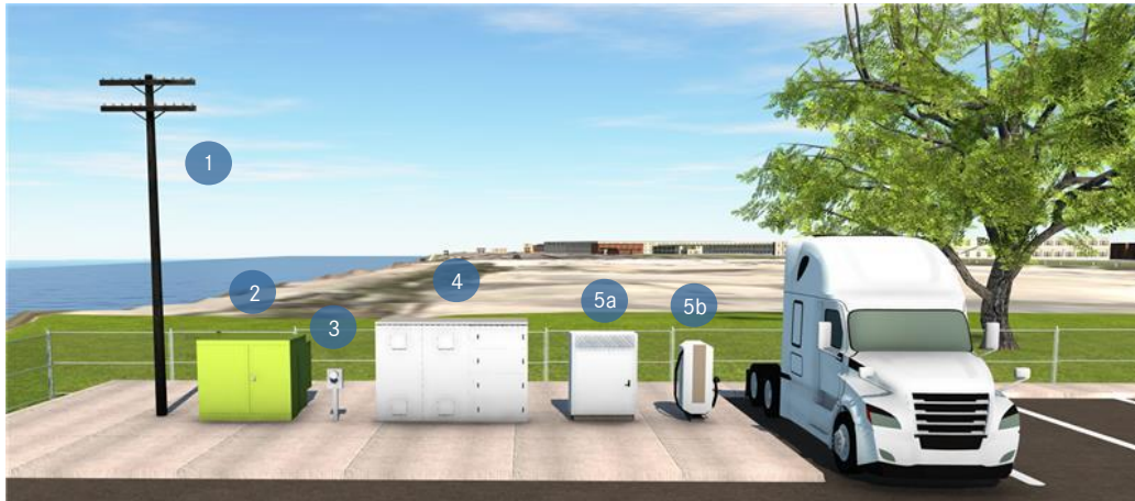
Figure 1. Illustration of Grid to Truck Energy Flow. (1) Power is pulled off primary voltage distribution lines, (2) voltage is stepped down over the transformer, (3) the meter measures how much energy is consumed, (4) the switchgear protects and isolates electrical equipment, (5a) the conversion unit (housed independently here) converts AC to DC and can sometimes be housed inside the dispenser, (5b) the dispenser connects to the vehicle via a CSS connector.
