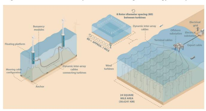
Figure 3: Schematic of an Example Full-Scale Floating Wind Energy Development
