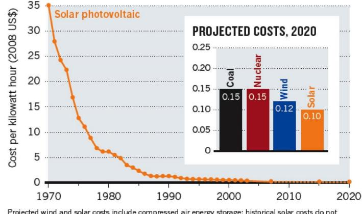
Projected wind and solar costs include compressed air energy storage; historical solar costs do not. Coal cost includes carbon capture and sequestration. Nuclear subsidies not included.
