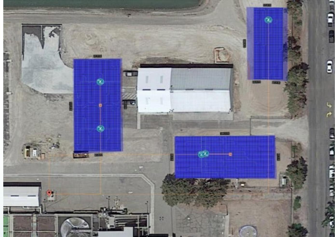
*Photo: Proposed Wastewater Treatment Plant PV System Layout*
