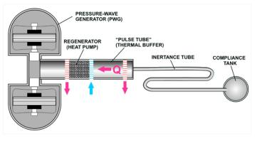
Figure 4: Simplified diagram of a thermoacoustic cryocooler
