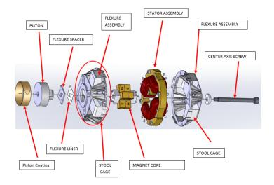
Figure 5: Basic components of a RIX linear motor
