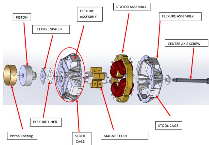
Figure 5: Basic components of a RIX linear motor
