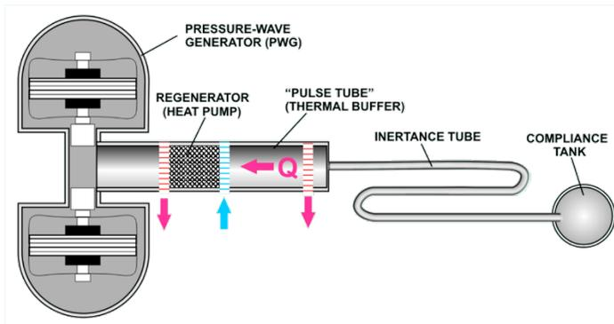
Figure 4: Simplified diagram of a thermoacoustic cryocooler
