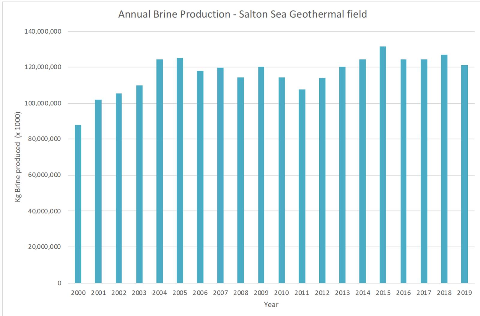
For the **current field's (400 MWe)** brine production rates: the total amount of Li contained in produced brine over a year = 120,000,000 kt x 0.0002 (200 ppm Li) = **24,000 tons Li metal/yr @ 400 Mwe**, equivalent to **128,000 tons LCE/yr @ 400 MWe**.
