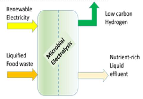
Figure: Microbial Electrolysis Process
