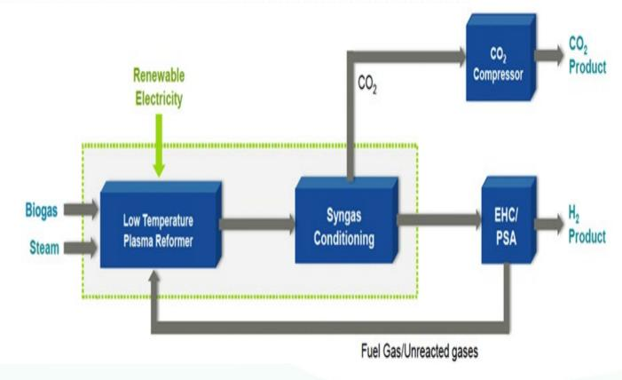
Figure: Catalytic Non-Thermal Plasma Reactor Process
