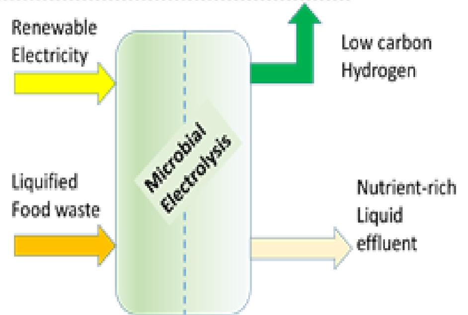
Figure: Microbial Electrolysis Process
