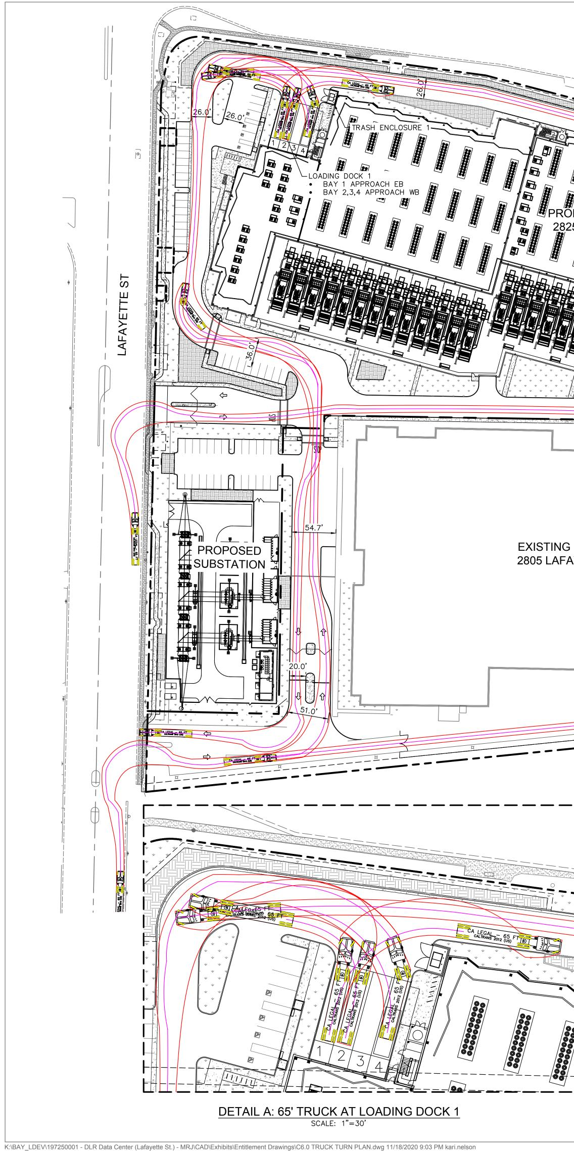
CENTRAL EXPRESSWAY SANTA CLARA COUNTY RIGHT OF WAY LOADING DOCK 2 **EXISTING BUILDING** 2805 LAFAYETTE ST LOADING DOCK 3-CALIFICAL - 65 FTTE - 31 \* \* \*0 \* \* \* GRAPHIC SCALE IN FEET 60 M 45.00 /@@ 3.00 20.00 CA LEGAL - 65 FT Tractor Width Trailer Width Tractor Track Trailer Track : 8.50 : 8.50 : 8.50 : 8.50 Lock to Lock Time Steering Angle Articulating Angle : 6.0 : 26.3 : 70.0 CA LEGAL - 65 FT DETAIL DETAIL B: 40' TRUCK AT LOADING DOCK 2 SCALE: 1"=30'
