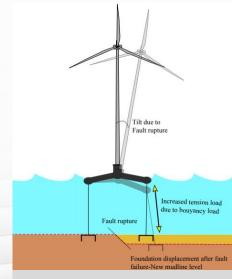
Effect of fault rupture on a floating offshore wind turbine supported by a tension leg platform
