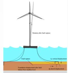
Effect of fault rupture on a floating offshore wind turbine with a catenary mooring system
