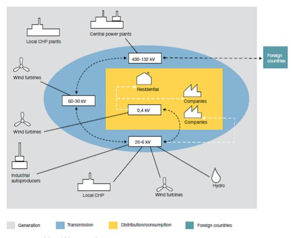
Figure 3: Structure of the grid in Denmark.
