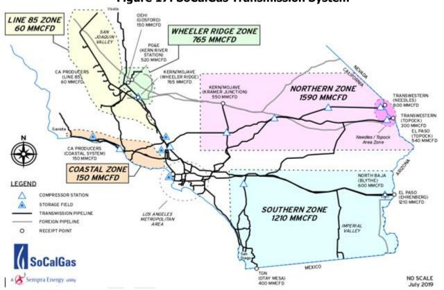
**Figure 17: SoCalGas Transmission System**
