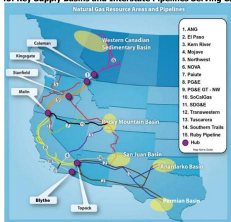
Figure 45: Key Supply Basins and Interstate Pipelines Serving California
