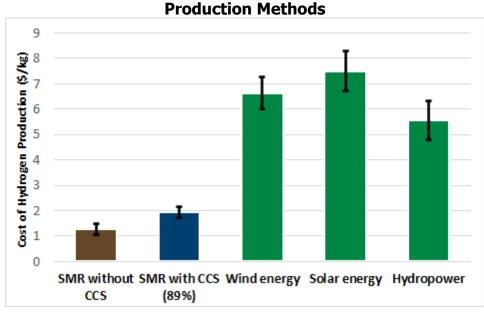
Figure 29: Cost of Hydrogen Production (\$/kilogram [kg]) of Selected Hydrogen
