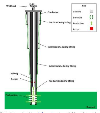
Figure 33: Wellhead, Production Casing, and Tubing Illustration
