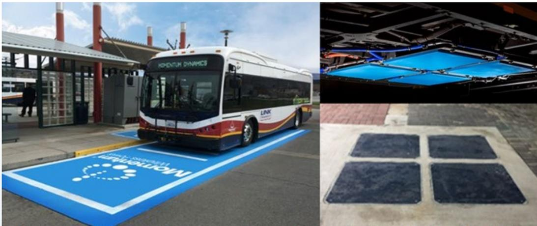
FIGURE 1: MD CHARGING SYSTEM IN-FIELD WITH CLOSE-UPS OF VEHICLE AND GROUND ASSEMBLY
