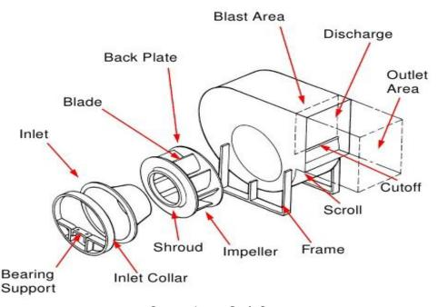
Figure 3-16: Centrifugal Fan Parts
