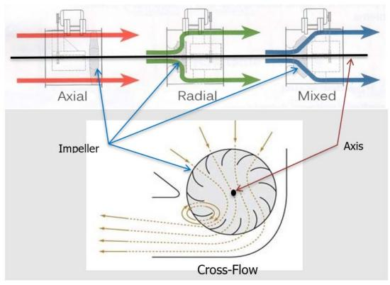
Figure 3-1: Axial-Flow, Radial-Flow, Mixed-Flow, and Cross-Flow
