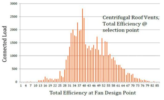
Figure 8-2: Centrifugal Power Roof Ventilator Fan Selection
