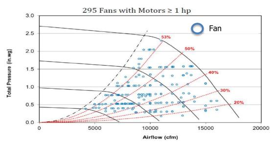
Figure 8-3: Fan Selection of Centrifugal Inline Fan Model
