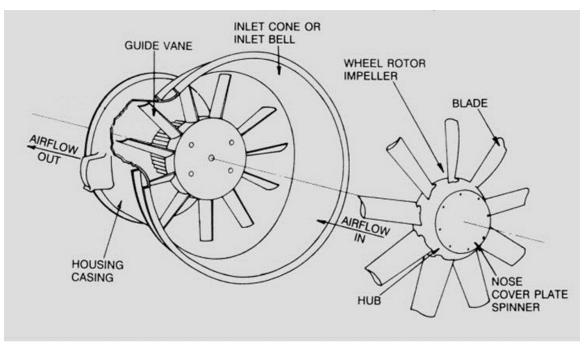
Figure 3-15: Vane-Axial Fan, Exploded View
