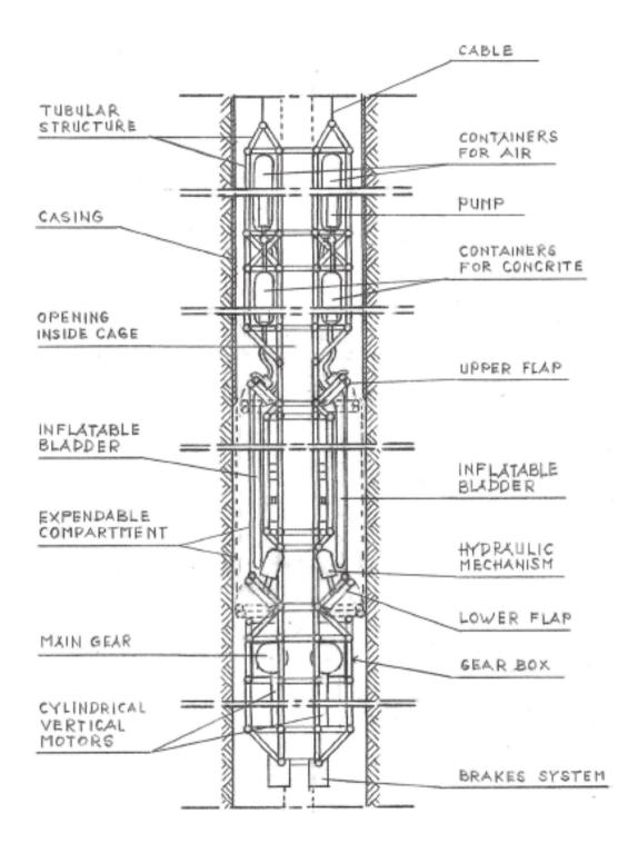
FIG. 7 - Cross-sectional view of a circular cage to be assembled on the excavation line of the apparatus for drilling faster, deeper, and wider wellbore.
