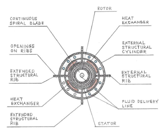
FIG. 6 - Cross-sectional view of an excavation line of the apparatus for drilling faster, deeper, and wider wellbore.
