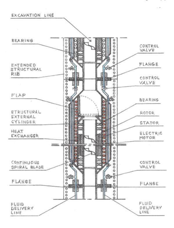
FIG. 5 - Cross-sectional view of an excavation line of the apparatus for drilling faster, deeper, and wider wellbore.
