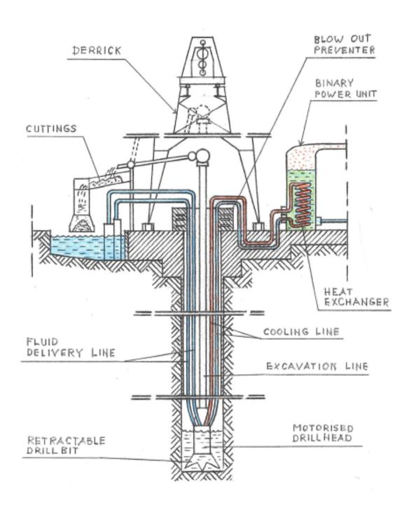
FIG. 1 - Schematic view of an apparatus for drilling faster, deeper, and wider wellbore.
