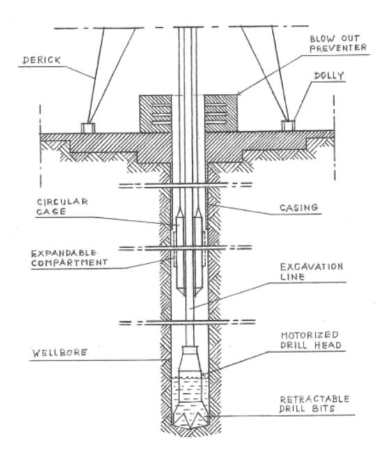
FIG. 2 - Schematic view of an apparatus for drilling faster, deeper, and wider wellbore with cage for casing.
