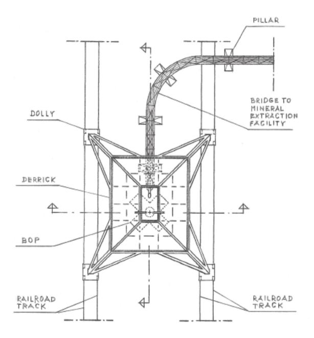
FIG. 4 - Plain cross-sectional view of an apparatus for drilling faster, deeper and wider wellbore.
