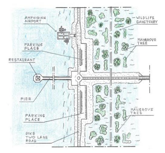
FIG. 7 – Plain view of a typical dike-pier intersection
