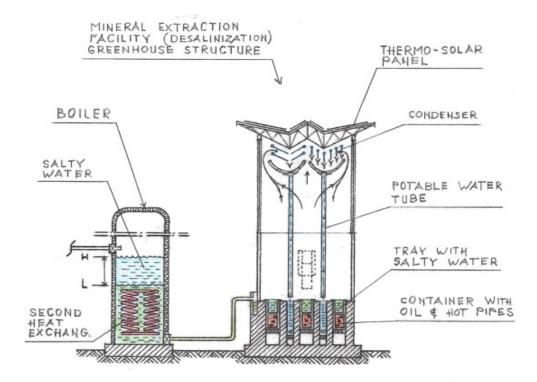
FIG. 17 – Schematic Cross-sectional View of a Power Plant for Desalinization of the Salton Sea, Production of Electricity, Potable Water, and Lithium
