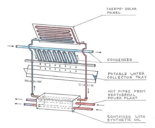
FIG. 18 – Perspective Cross-sectional View of an alternative Thermo-Solar System used in Desalinization Plant
