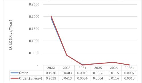
Figure 24: Loss of Load Expectation Comparison for Energy Limited Cases
