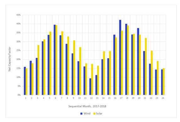
Figure 4: Capacity Factors by Month During 2017 and 2018
