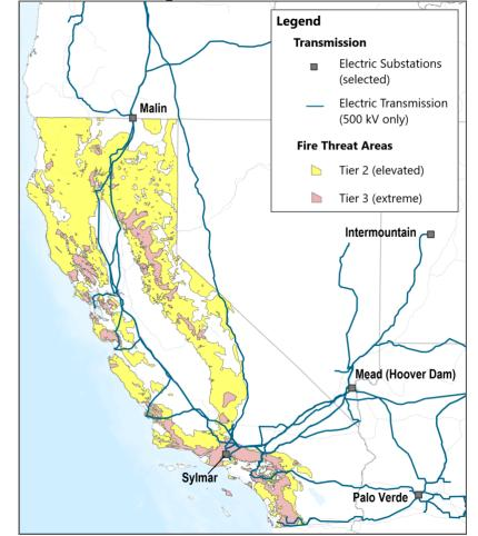
Figure 18: California-Serving 500 kV Transmission and In-State Fire Risk
