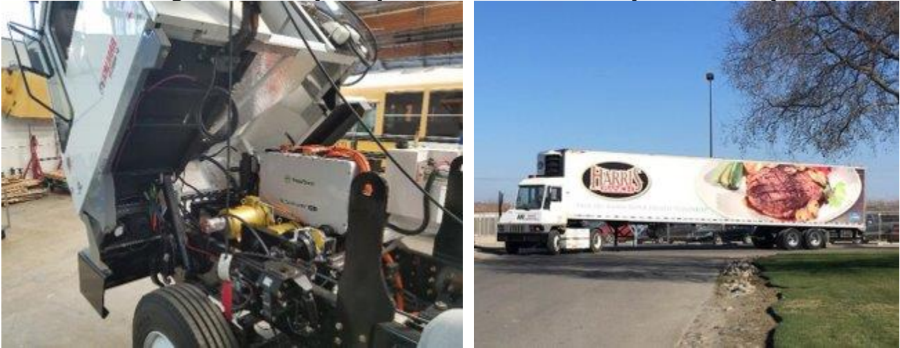
Figure 5: Heavy-Duty Electric Yard Tractor (TransPower)
