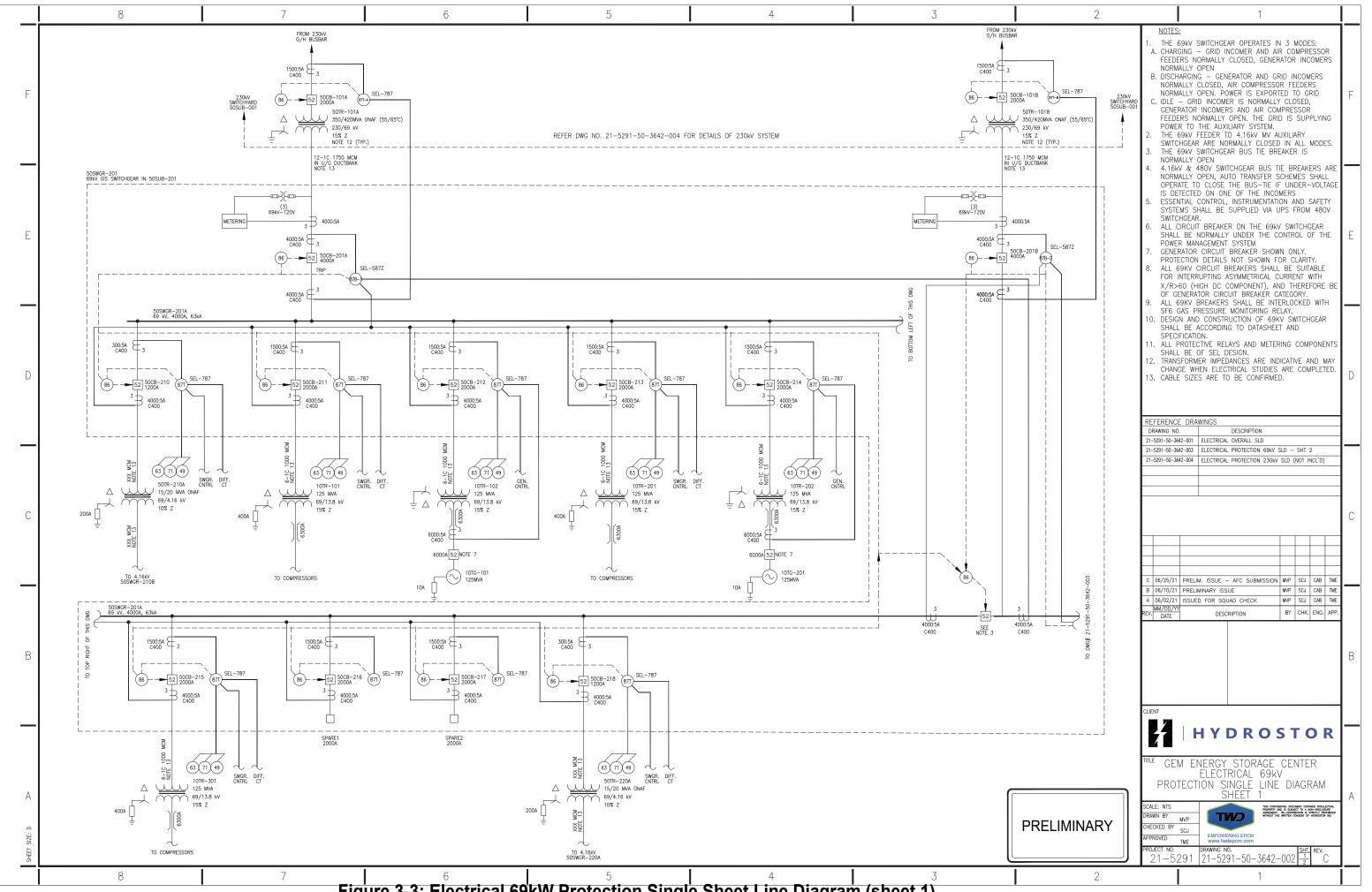
Figure 3-3: Electrical 69kW Protection Single Sheet Line Diagram (sheet 1)
