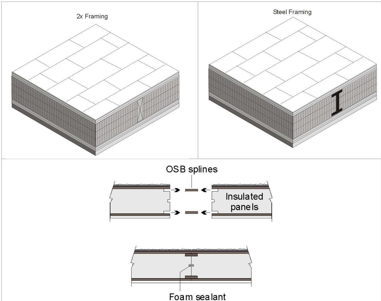
Figure 4.2.3 – SIPS Roof/Ceiling
