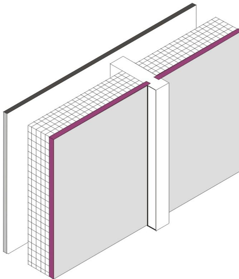
Figure 4.3.8 – Spandrel Panel
