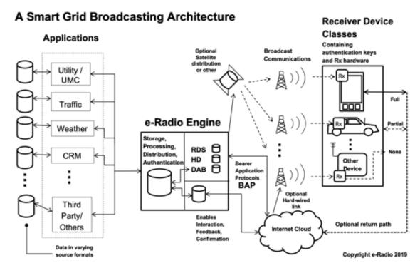
Figure 2. Hybrid IP+FM data architecture
