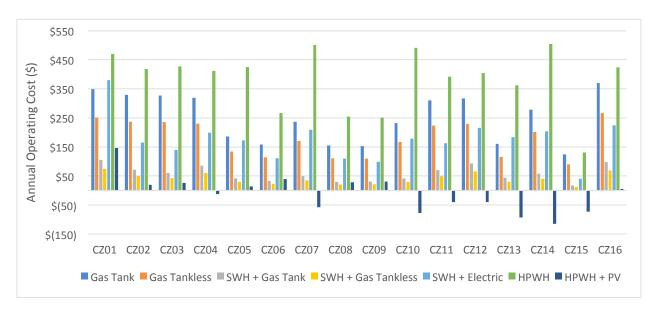
Figure 20. Annual operating costs for residential water heater configurations.
