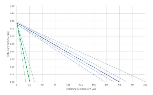
Figure 27. SRCC OG-100 collector efficiency curves for glazed selective surface (blue) & unglazed polymer (green) under full sun (1000  $W/m^2$ ). Individual sample collectors are shown as light solid lines. Average collector performance used in simulations is illustrated by the thick dashed lines.
