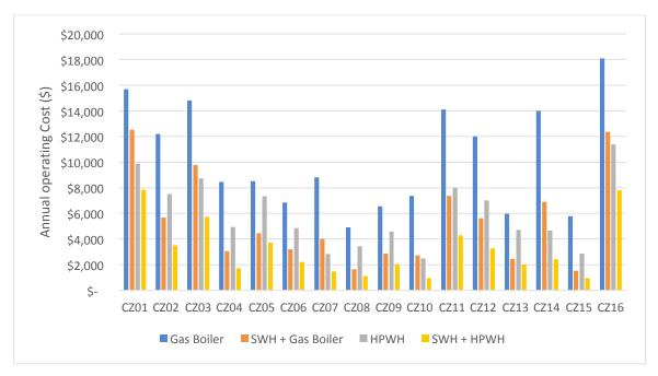
Figure 24. Annual operating costs for commercial pool heating configurations.
