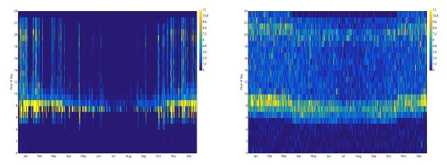
Figure 31. Heat maps of energy use for multifamily solar thermal system (left) and heat pump (right) in Climate Zone 3 (San Francisco). Legend is scaled with a peak of 12 kW.
