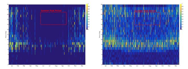
Figure 30. Heat maps of residential electricity use for solar thermal system (left) and heat pump (right) in Climate Zone 3 (San Francisco). The summer peak TOU period is indicated. Legend is scaled with a peak of 1 kWh.
