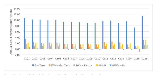
Figure 21. Annual GHG emissions for multifamily water heating configurations.
