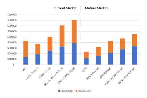
Figure 17. Current and mature market pricing for commercial pool technologies and configurations.
