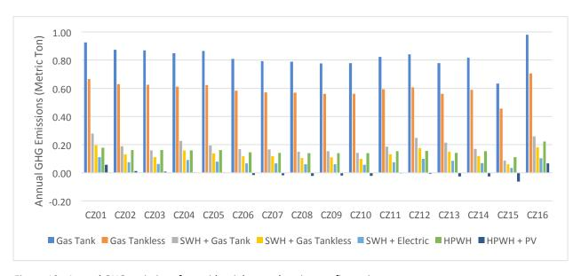
Figure 19. Annual GHG emissions for residential water heating configurations.
