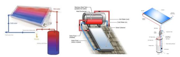
Figure 9. Common styles of solar water heating systems. Integral Collector Storage (left), thermosiphon (middle), active closed-loop (right).
