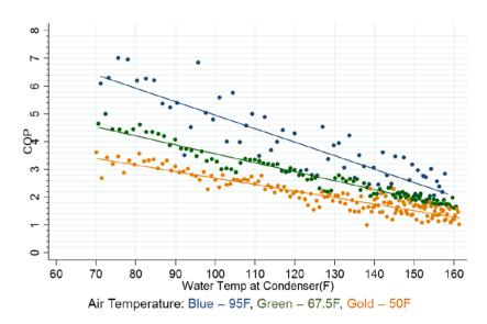
Figure 28. Heat pump efficiency (COP) as a function of water heater & environmental temperature (Carew et al. 2018).
