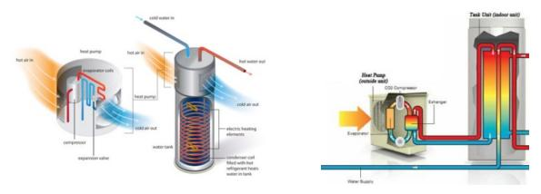
Figure 7. Residential HPWH system types present in US market. Cutaway diagrams of 'All-in-One' (left) & EcoCute™ 'split system' (right).
