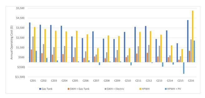
Figure 22. Annual operating costs for multifamily water heater configurations.
