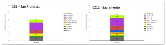
Figure 4. Breakout of carbon emissions by end use for 2,500 ft2 home in two California climate zones.
