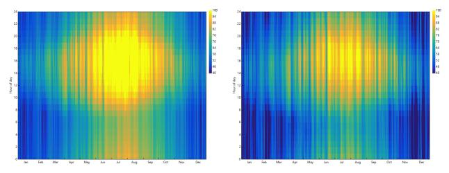
Figure 26. Heat pump environmental operating temperatures for garage (left) and outdoor air (right) in Climate Zone 16 (Tahoe region). The lower legend of 40 F indicates the limit of heat pump operation before backup resistance heating engages.
