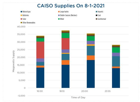
Figure B-3: California ISO Changing Resource Mix as Solar Generation Declined on August 1, 2021
