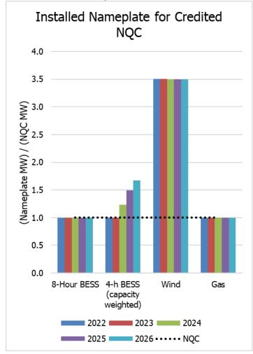
Figure 2: Comparison of the Nameplate Capacity Necessary to Provide 1 MW NQC of BESS, Wind and Gas
