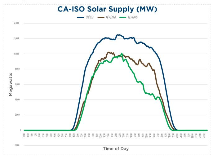
Figure B-2: Solar Output in California ISO on August 1, 14, and 31, 2021
