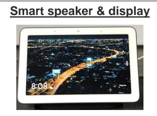
Voice activation: Prevent speech Ambient light sensor: Control ambient light (test at 10 lux and 300 lux)
