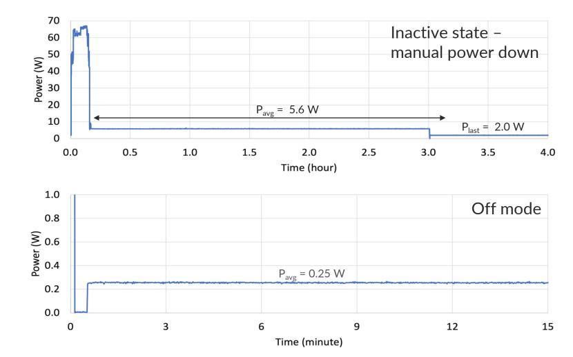
Example of additional tests for a game console: manual power down (top) and off mode (bottom). Preliminary data for illustration purposes only. Source: CA IOU Team.
