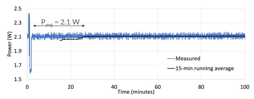
Example of test period for a connected smart home product that powers down to a pinging mode. Preliminary data for illustration purposes only. Source: CA IOU Team.
