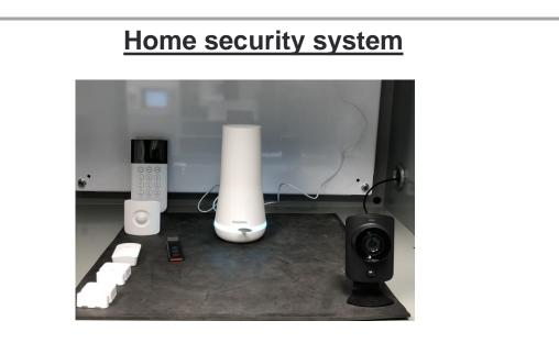
Connect base station and camera to 120Vac power Download and set up app Pair sensors and camera to base station Update software
