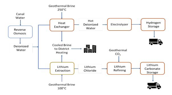
FIGURE 7.6 Conceptual design of lithium and hydrogen extraction from Salton Sea geothermal brines at temperatures of 250°C and 100°C. Direct conversion of lithium chloride to a lithium hydroxide product would be more advantageous for battery manufacture. Credit: Elders et al. (2019).
