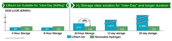
Figure 1. Cost of Energy Storage - Battery vs Hydrogen:
