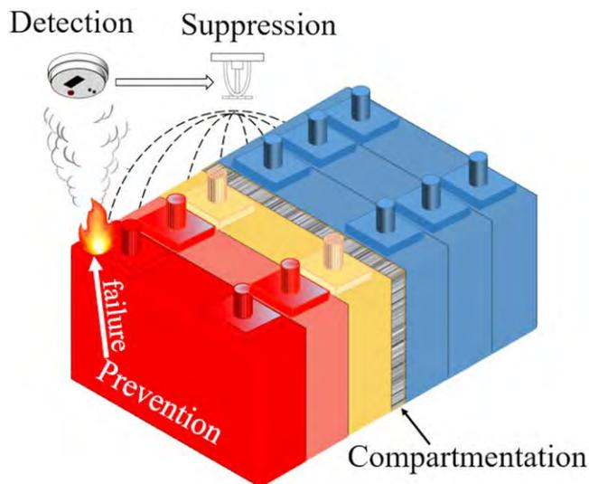
**Figure 2.** The four layers of fire protection present in LIB. Prevention includes safety components and safety devices. Once prevention fails, the detection layer can provide quick warning, triggering suppression and the emergency response. Compartmentation aims at delaying or stopping the propagation to other cells and modules.
