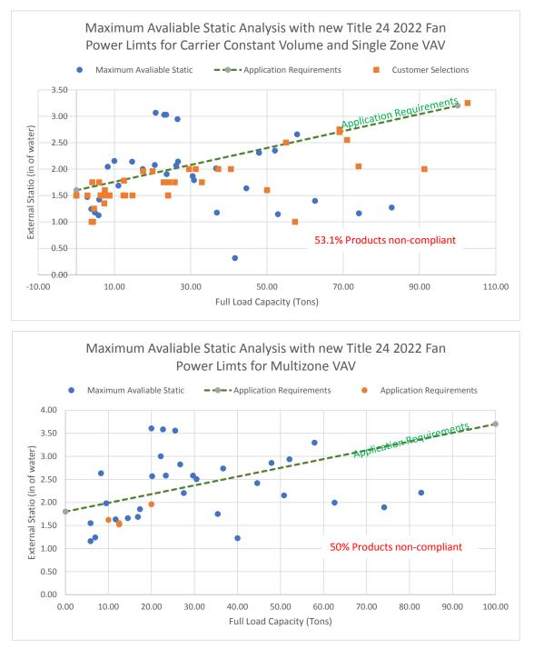
As you can see 53.1% of the CV units and 50% of the VAV would not even be able to provide the assumed customer requirements specification line.
