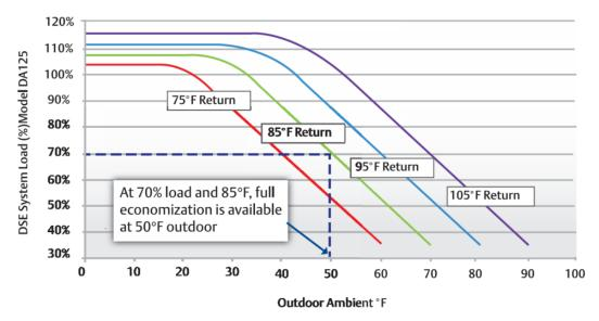
Figure 2. Manufacturer Data on Capacity Load Factor and Return Air Temperature's Impacts on Pumped Refrigerant Economizer CRAC
