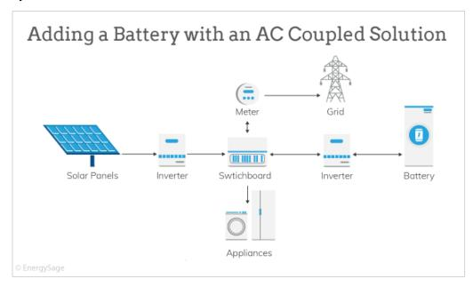
Figure 2: Battery storage system paired with solar PV.
