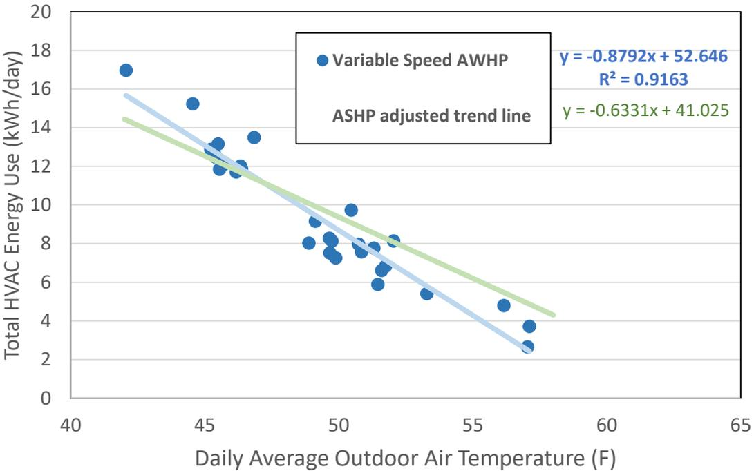
**Figure 7: Comparison of monitored variable speed AWP and model adjusted prescriptive ASHP heating energy use as a function of daily average outdoor air temperature.**
