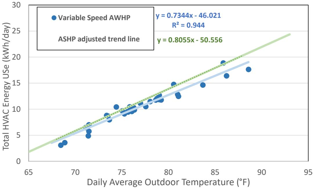
**Figure 6: Comparison of monitored variable speed AWP and model adjusted prescriptive ASHP cooling energy use as a function of daily average outdoor air temperature.**
