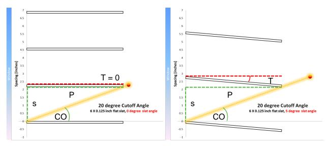
Figure 2: Cutoff angle, tilt angle, and projection factor.
