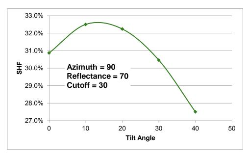
Figure 3: Shading factor as a function of tilt angle for a horizontal slat.
