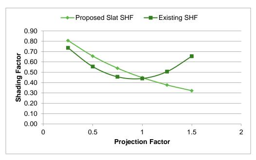
Figure 6: Comparison of the existing shading factor and proposed shading factor for a south-facing horizontal slat.
