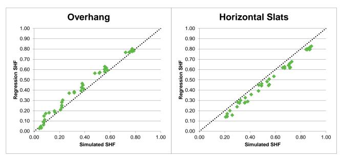
Figure 5: Shading factor regression curve versus simulated values.
