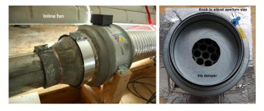
Figure 2. Inline fan and damper used to control air flows
