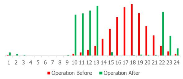
Figure 9: CBECC model results for AC load shifting
