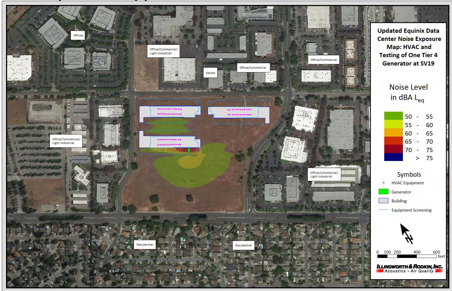
FIGURE 2 Noise Exposure Resulting from Testing of One Generator at Building SV19 at 100% Load Concurrent with Operation of HVAC Equipment
