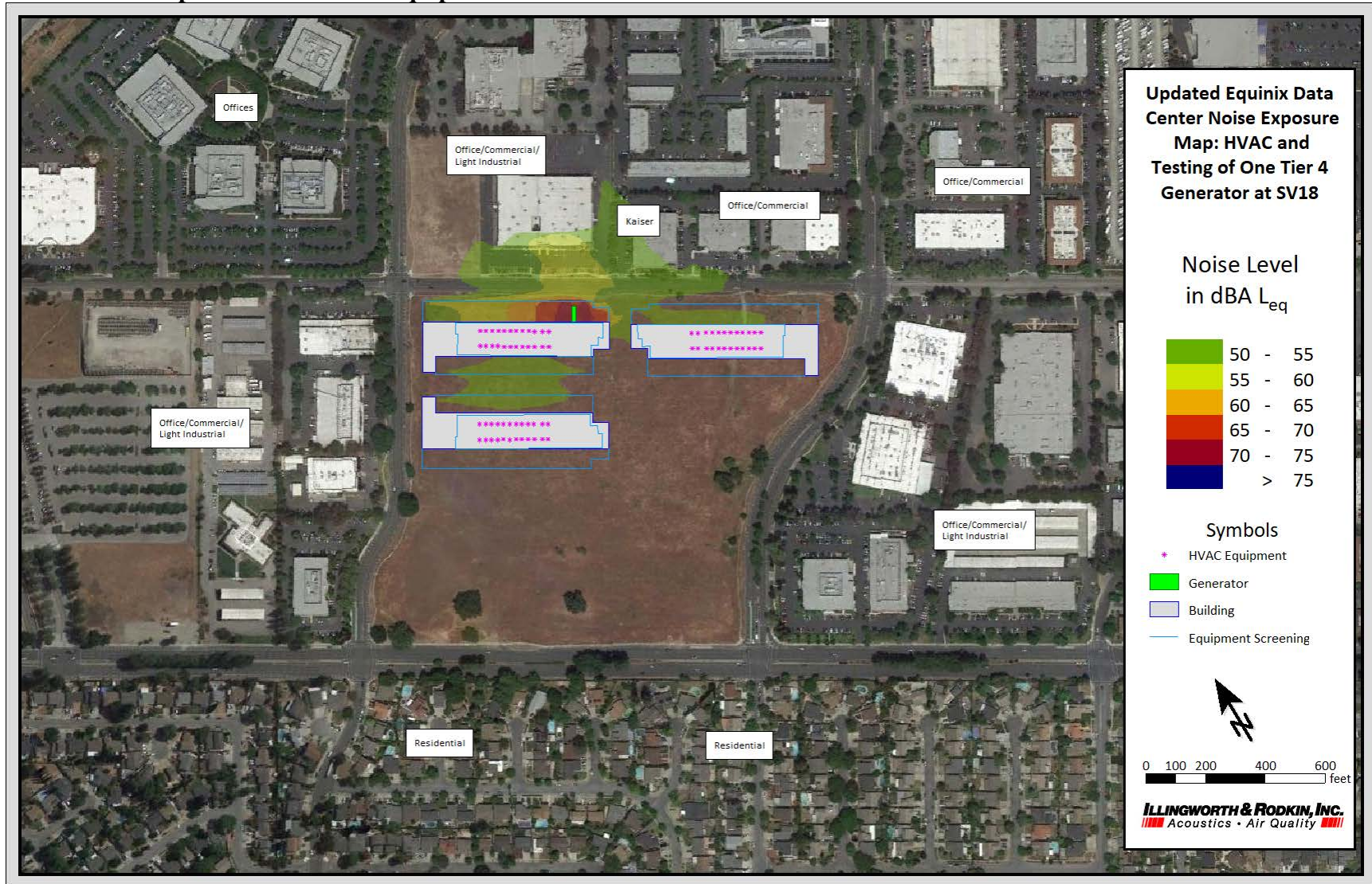
FIGURE 2 Noise Exposure Resulting from Testing of One Generator at Building SV18 at 100% Load Concurrent with Operation of HVAC Equipment
