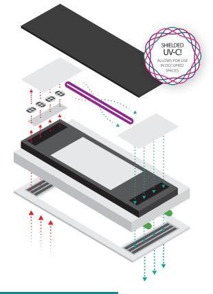
UV-C technology has been used as a disinfection method for decades. The UV-C wavelength of 253.7 nanometers has been proven to be effective at neutralizing dangerous microorganisms. The challenge with UV-C technology has always been the method of delivery. It can't be used in occupied spaces and is only effective on direct line of sight areas. Until now!
