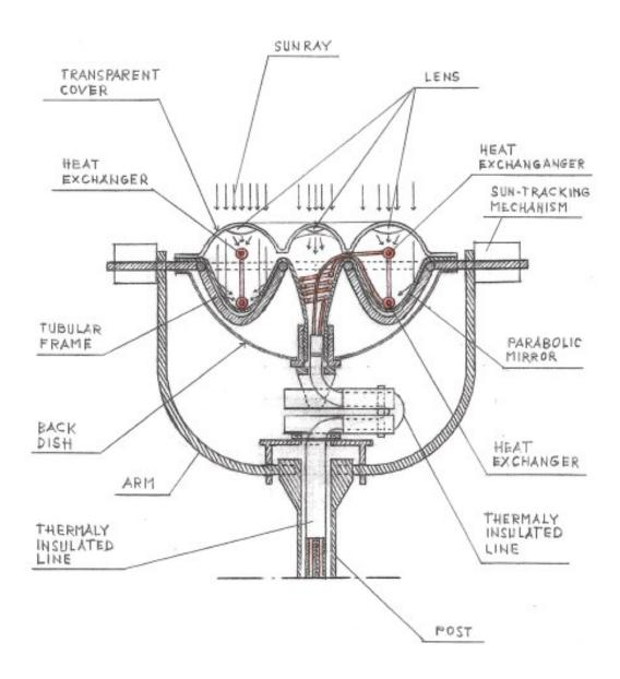
FIG. 3 - Cross-sectional View of the "Thermo - Optical Solar Dish"
