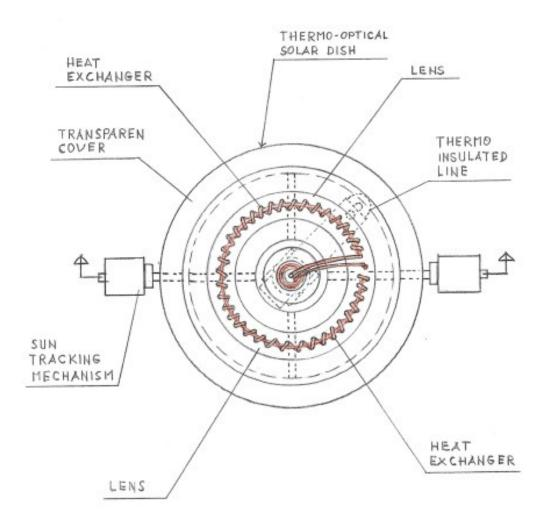
FIG. 4 - Plain View of a "Thermo-Optical Solar Dish"
