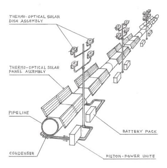
FIG. 1 - Perspective View of a Pipeline with Solar Panels
