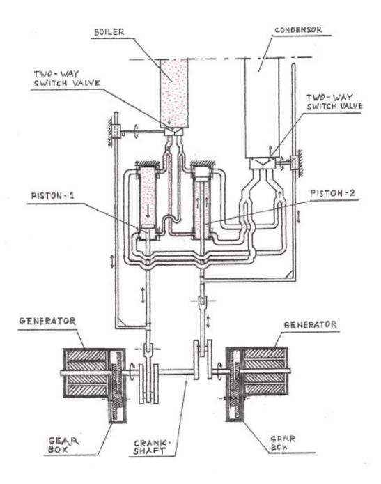
FIG. 8 - Schematic Diagram of a Piston Power Unit - stroke one
