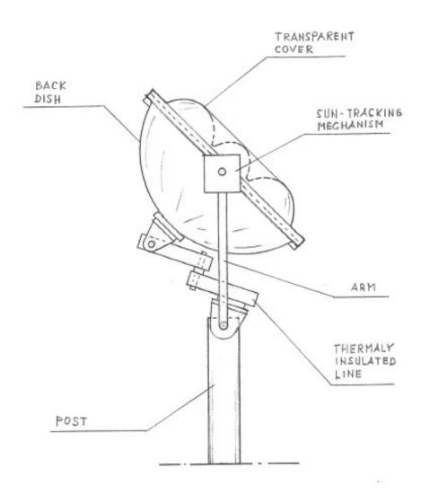
FIG. 5 - Side View of a "Thermo-Optical Solar Dish{"
