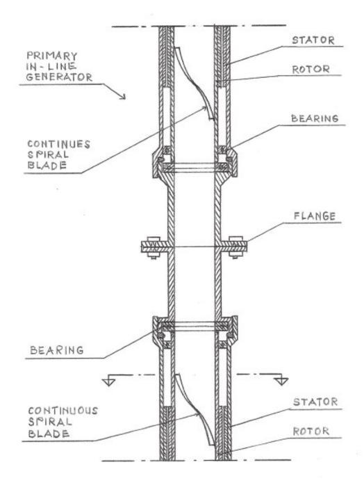
FIG. 6 – Cross-sectional longitudinal View of the Primary In-Line-Pump / Generator
