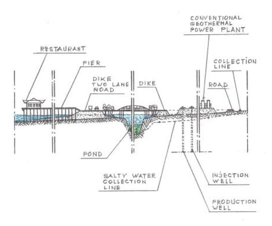
FIG. 6 – Cross-sectional view taken near a typical dike-pier intersection
