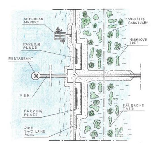
$\pmb{FIG. 7} - \textbf{Plain view of a typical dike-pier intersection}$
