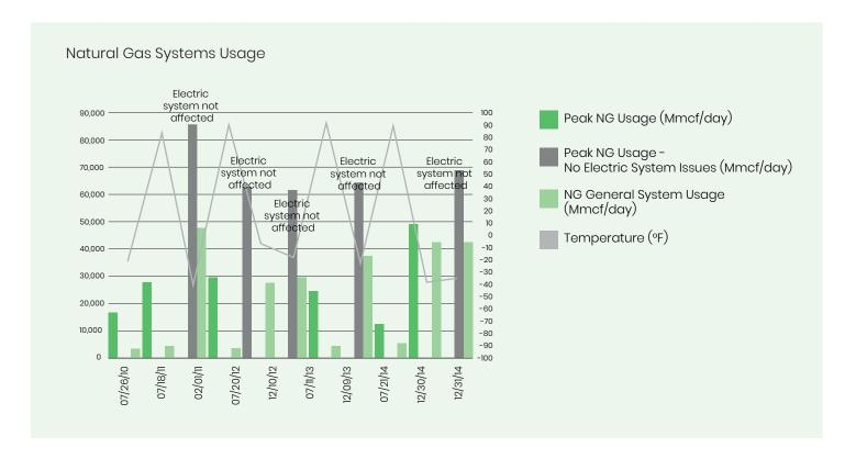
Correlated failure between the natural gas grid and the electric grid has an estimated likelihood of 1.5% for outages over 36 hours. In comparison, diesel resupply failure is 14% at 36 hours,
