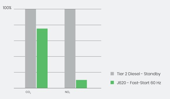
The Jenbacher J620 fast-start, natural gas generator without after treatment technologies can provide an emission reduction of up to 23%  $\rm CO_2$  and up to 90%  $\rm NO_x$  compared to Diesel Tier 2 standby generators.
