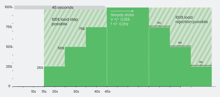
1. Example profile for pre-heated/-lubricated; Without synchronization; 480 V configuration; Power quality within +/- 10% voltage, +/- 5% frequency
