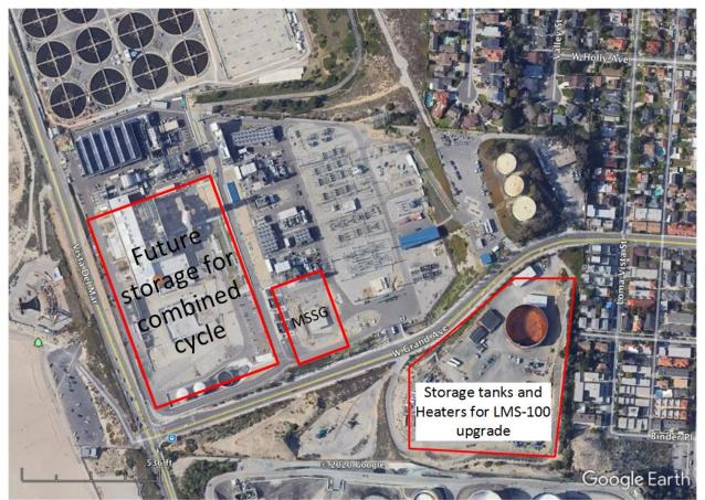
Figure 5. Scattergood Generating Station aerial view. The rectangular area including the boiler house and turbine hall for Units 1-3 and adjacent vacant land, is approximately 750 feet x 500 feet, and could be used for about 10 GWh of energy storage to support the existing combined cycle.
