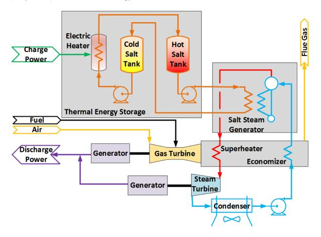
Figure 1. The patented Liquid Salt Combined Cycle (LSCC) integrates proven equipment in a novel system to create technical, economic and operational synergies.
