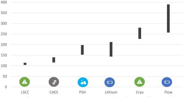
Figure 11. Bulk storage systems have the lowest Levelized Cost of Energy at 8-hours and above for 100MW capacity. Liquid Salt Combined Cycle technology is the cost leader.<sup>3</sup>
