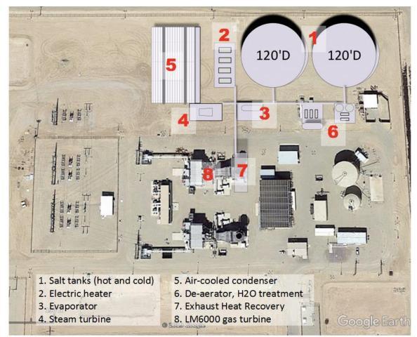
Figure 3. Conceptual general arrangement showing the upgrade of one out of two units at an existing peaking plant.
