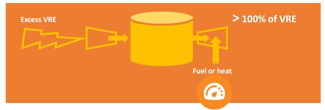
Figure 10. Hybrids use fuel or heat to boost the performance and reduce the cost of energy storage
