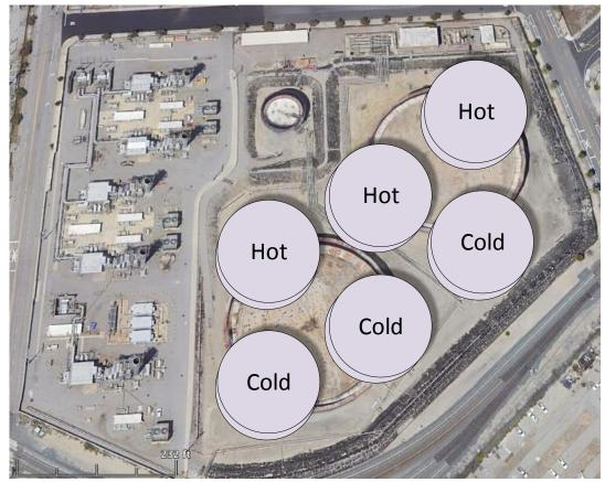
Figure 4. An 11,000 MWh energy storage system could be deployed at Harbor Generating Station, using six molten salt storage tanks, similar in design and construction to the 12 tanks installed at the Solana CSP station in Arizona. Similar systems could also be installed at the Scattergood and Haynes Generating Stations.
