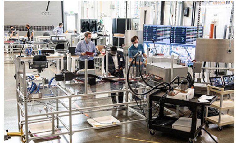
Researchers evaluate megawatt charging connector systems on the liquid-cooled (near) and air-cooled (far) test-benches. Photo by Dennis Schroeder, NREL
