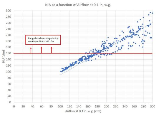
**Figure 1.** NIA as a function of rated airflow at 0.1 in. w.g. (estimated based on preliminary calculations). This chart shows an excerpt of the full range of range hoods listed in HVI's CPD database; hoods with airflows beyond the maximum values shown in the figure are not included here. This figure is provided
