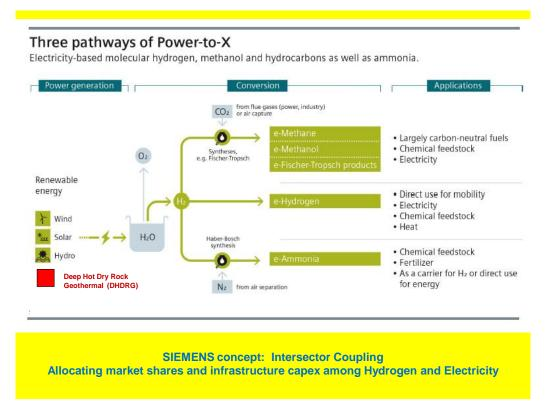
Figure 19. Hydrogen's role in "Inter-sector" or "Cross-sector" coupling: concepts for exploring definitions for [ energy + feedstocks ] systems for the entire human enterprise, before year 2050. Save otherwise-curtailed wind and PV in CA ?
