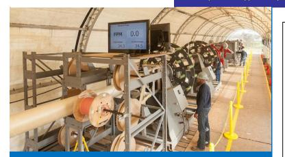
Smart Pipe Company, Houston **On-site pipeline factory Continuous process, unlimited length** Hydrogen-compatible: polymer-metal hybrid resists HE, HCC
