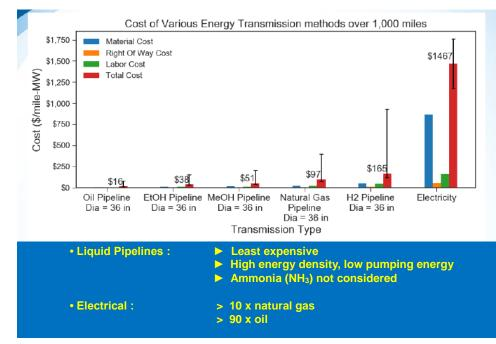
Figure 12. From research supported by an award from the Department of Energy (DOE) Office of Energy Efficiency and Renewable Energy under Award Number DE- EE0007602 and by Alliance for Sustainable Energy, LLC, the manager and operator of the National Renewable Energy Laboratory for the U.S. Department of Energy (DOE) under Contract No. DE-AC36-08GO28308. (Unpublished at 17 Aug 20, but submitted to one or more journals by the authors)
