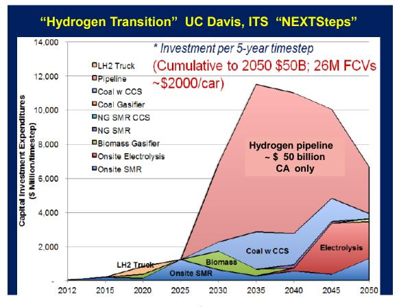
Figure 5. From "The Hydrogen Transition", ITS-STEPS, 2014<sup>1</sup> Large cumulative capex for "Hydrogen Pipeline" if building a new, dedicated, high-purity, underground GH2 pipeline system; less capex if diverse extant pipelines are repurposed.
