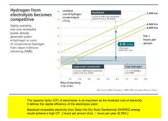
Figure 21. Hydrogen's role in "Inter-sector" or "Cross-sector" coupling: prospects for profitably harvesting otherwisecurtailed wind and solar energy, in CA and beyond, because of low CF of electrolysis and hydrogen gathering assets.
